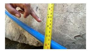
Figure 3.1. Measuring of Maximum Flood Height.
